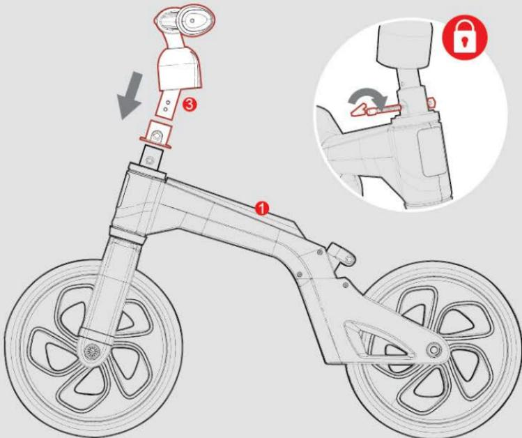
EN: Do not over tighten the screws as it may cause damage to the trike.
