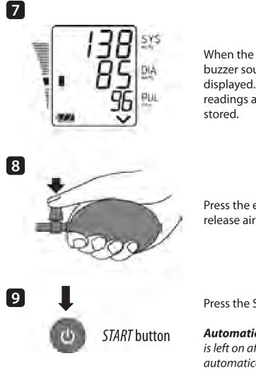
When the measurement is complete, the buzzer sounds and the ✔ mark is displayed. The systolic and diastolic pressure readings and pulse rate are displayed and stored.
