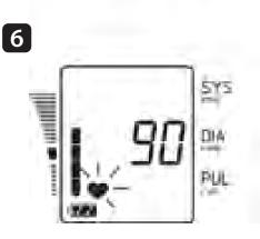
The deflation starts automatically. The heart mark  $\clubsuit$  starts blinking, indicating that the measurement is in progress.
